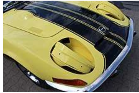
Opel GT with headlights turned up When turning, both headlights turn in the same direction
